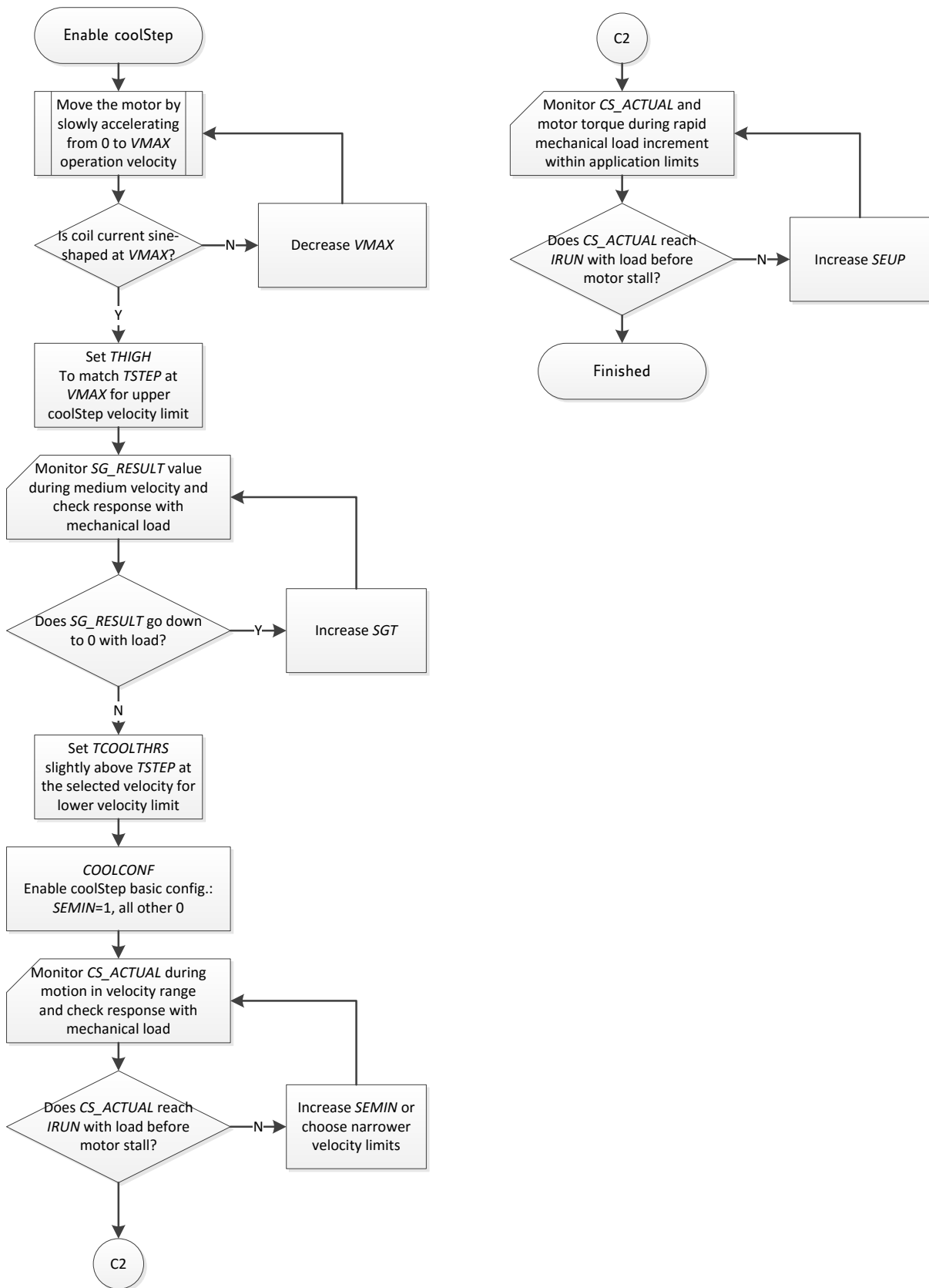
Figure 24.4 Enabling coolStep (only in combination with spreadCycle)
